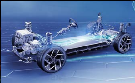
Safety - E-Platform 3.0 With The Cell-to-Body (CTB) Structure
